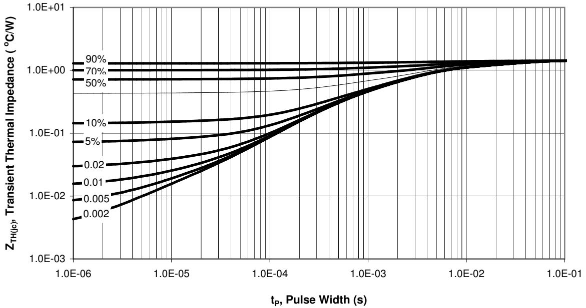
Figure 7. Transient Thermal Impedance Z_{th(jc)} = f(t_p) ; parameter: Duty Ratio
