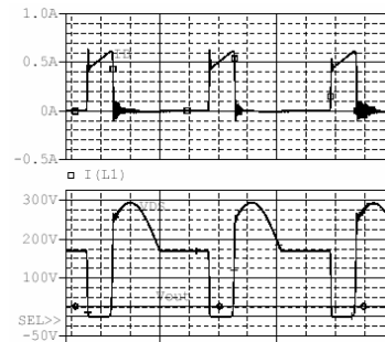
Figure 4b. Simulation results. V_{\text{in}} = 170 \text{ V} , V_{\text{out}} = 24 \text{ V} , f_s = 50 \text{ kHz} .
